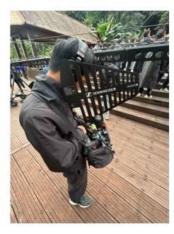
Xu Mengyu modified the antenna of one of the receivers recording the backup track into a passive directional model. This further enhanced the signal reception range, increasing signal stability in an extremely complex environment
